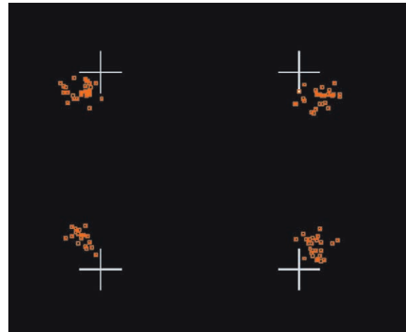
Add impairments or correct baseband deficiencies by adjusting I/Q gain, dc offset and quadrature skew.
